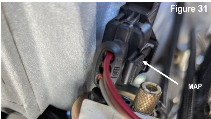
MAP: Connects to the manifold absolute pressure (MAP) sensor mounted on the rear of the manifold.
